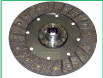
Clutch driven plate Studebaker Weasel M29C HDS-57
