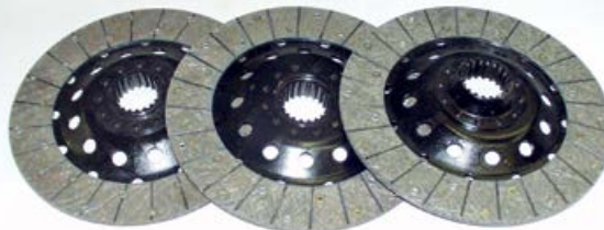
DRIVING PLATES HDS 57 M131 „HURVÍNEK“ railway vehicle
